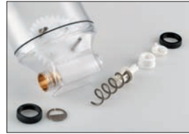
Portion controller with individual parts, dosing auger
